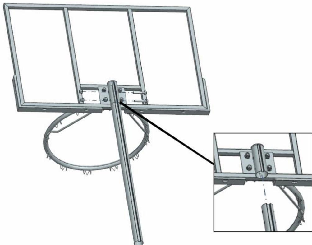
**Connect the upper rod (11), middle rod (3), and lower rod (6) together and tighten them with a knob**
