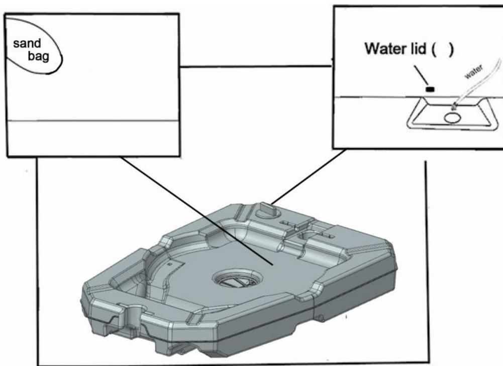
**For safety reason, sand instead of water is recommended to fill up the base during the sub-freezing weather. Please note that sand will not be poured out once filled in the base**
